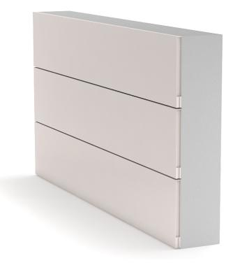
Conceptual view of the thin panel placed on a rigid wall with one layer of square cross-section Helmholtz resonators. Credit: CNRS
