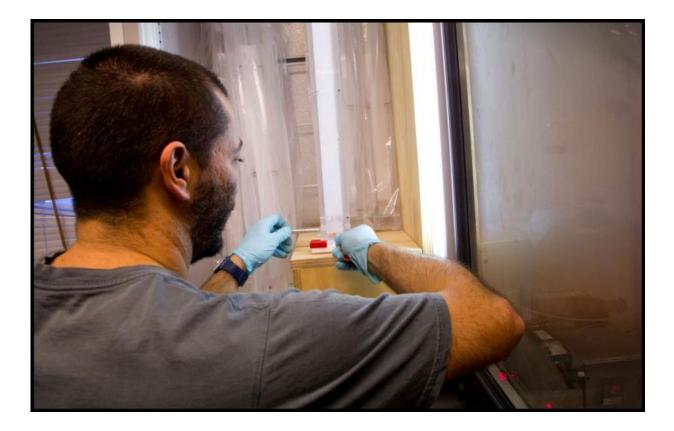
The ice is cut out and melted on a warm melting head. The new method measures the meltwater directly and the data can already be analysed a few seconds after melting the ice. Credit: Ola Jakup Joensen, NBI
