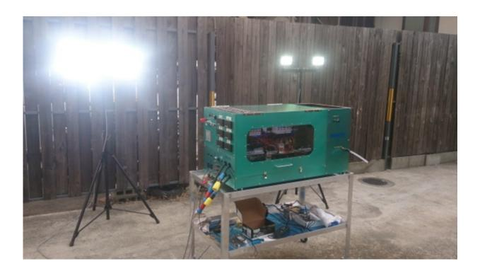
Small jet engine generator equipped with ZnO-coated bearings for emergency use (Lights in the back are being turned on using the power produced by the generator). Credit: NIMS
