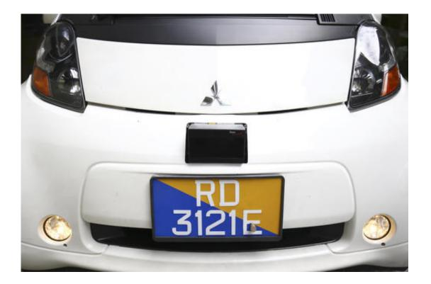
A "lidar" that detects obstacles using laser sensors is installed above the car plate of an autonomous vehicle during its test drive in Singapore Wednesday, Aug. 24, 2016. The world's first self-driving taxis, operated by nuTonomy, an autonomous vehicle software startup, will be picking up passengers in Singapore starting Thursday, Aug. 25. The service will start small - six cars now, growing to a dozen
