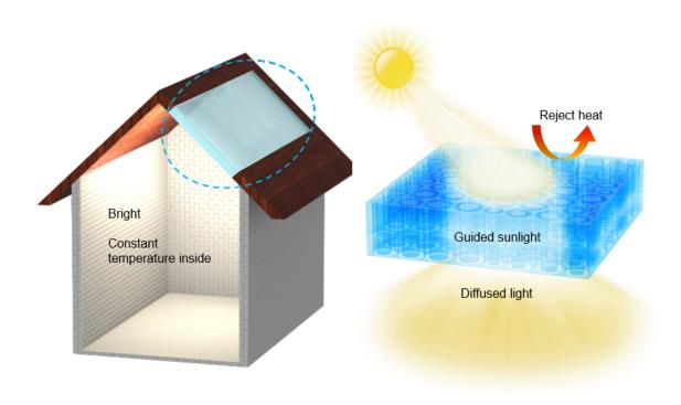
A wood composite as an energy efficient building material: Guided sunlight transmission and effective thermal insulation. Credit: University of Maryland and Advanced Energy Materials
