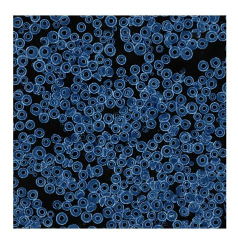
A microscopic image of doughnut-shaped microparticles, made from silica nanoparticles through vortex ring freezing. This work is detailed in a paper published on Aug. 4 in *Nature Communications*. Credit: Cornell University
