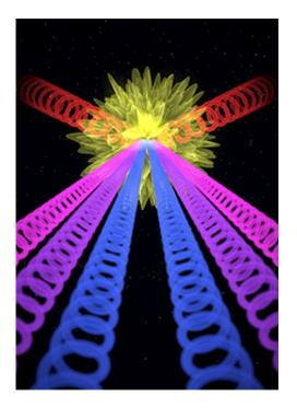
Counter-rotating circularly polarized laser beams (red) are crossed in a gas target to generate angularly separated extreme ultraviolet (EUV) harmonics with rightand left-circular polarization (blue, purple, magenta). This method provides straightforward and robust control of the direction, polarization, and spectrum of the light, opening the door to investigating materials in ways that were never before possible. Credit: US Department of Energy
