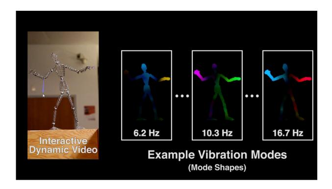
To simulate objects, researchers analyzed video clips to find "vibration modes" at different frequencies that each represent distinct ways that an object can move. By identifying these modes' shapes, the researchers can begin to predict how these objects will move in new situations. Credit: Abe Davis/MIT CSAIL
