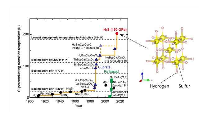
(Left) Development of the superconducting transition temperature Tc. Hydrogen sulfide's highest Tc is  $H_2S$  (150 GPa), and this is 30 K higher than what was previously the highest Tc superconductor  $\hat{a} \in \Phi$  Cuprate, Hg-Ba2Ca2Cu3Oy - and the lowest temperature ever recorded on the Earth's surface to date (184 K/-93 $\hat{a}$ ,  $\Phi$ ). Credit: Osaka University
