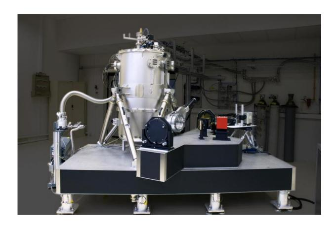
Hexapods are used to align the French MIRIM imager, one of four infrared instruments for the James Webb Space Telescope, an international astronomical mission involving NASA and ESA. Credit: Symetrie/CEA
