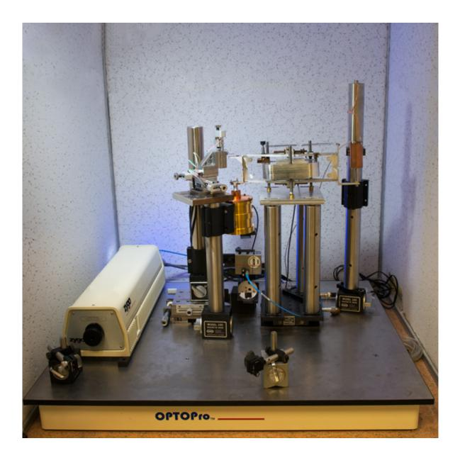
An early prototype of the Electrostatic Force Balance (EFB). The gold-colored cylinder (center) is the capacitor. Applying a force to the balance causes the rectangular flexure (center, right of capacitor) to move. The inner electrode of the capacitor (copper-colored cylinder) is attached to the flexure. Credit: National Institute of Standards and Technology
