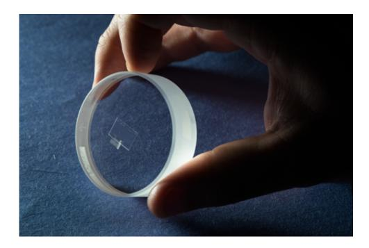
PML researcher Gordon Shaw holding a prototype for the chip-sized small-force meter. The cantilever is near the intersection of the two rectangles in the center of the glass cylinder. Credit: National Institute of Standards and Technology
