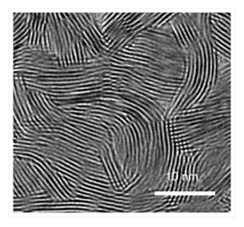
An electron micrograph shows the pattern of nanostructured walls on the surface of the device. Plopped into a sample of contaminated water and placed in sunlight, it killed more than 99.999 percent of bacteria in just 20 minutes. Credit: C. Liu et al., Nature Nanotechnology
