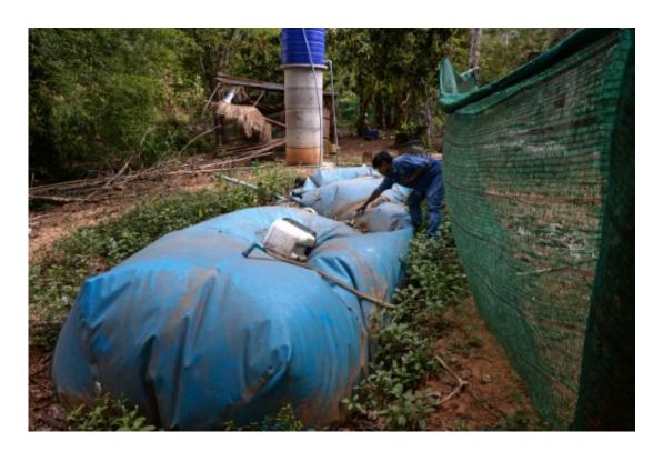
Balloons fill up with methane gas after microbes break down the animal manure and other organic waste packed inside
