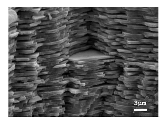
Electron microscopy image of a fractured surface of nacre. Credit: Fabian Heinemann/Wikipedia
