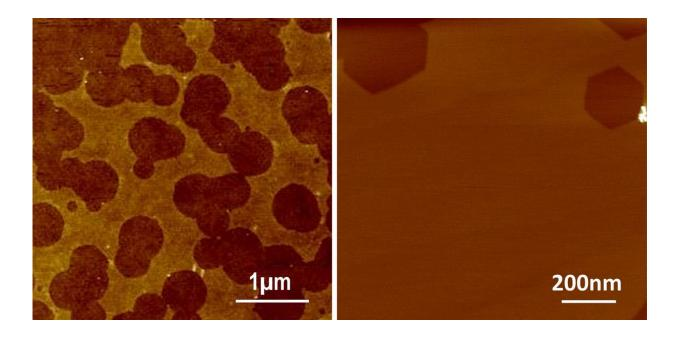
Graphene etched with an underlying silica substrate produces uneven edges (figure 1) but forms precise edges when placed on boron nitride (figure 2). Credit: Guangyu Zhang
