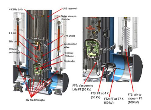
The Medium Scale High Voltage Test apparatus in TA-53 Building 10 allowed scientists to test electric fields in liquid helium, a crucial part of upcoming experiments into the nature of matter and antimatter. Credit: Los Alamos National Laboratory
