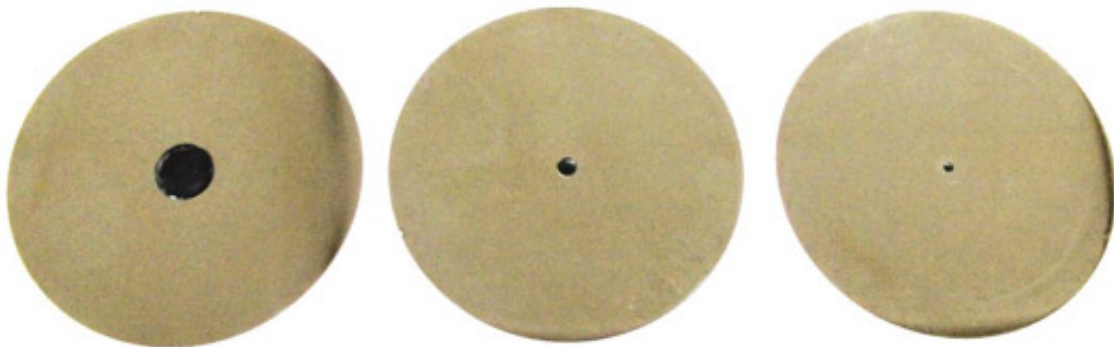
Figure 1: The reverse sides of three standard gas barrier (SGB) films developed WVTR 1.0 \times 10^{-4} g m -2 day -1 (20 mm in diameter of the hole)(left), 1.1 \times 10^{-5} g m -2 day -1 (6.5 mm in diameter)(center), 3.1 \times 10^{-6} g m -2 day -1 (3.5 mm in diameter)(right). Credit: Advanced Industrial Science and Technology
