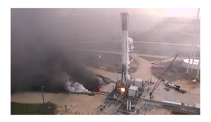
SpaceX completed the first full duration test firing of a landed first stage booster on July 28, 2016 on a test stand at their rocket development facility in McGregor, Texas. Credit: SpaceX
