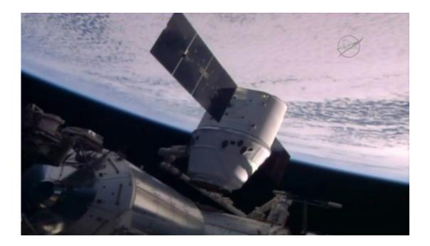
SpaceX's Dragon, pictured on July 20, 2016 at the International Space Station, is the only cargo carrier in use that can return gear to Earth. Others, such as Orbital ATK's Cygnus, burn up on re-entry to Earth's atmosphere
