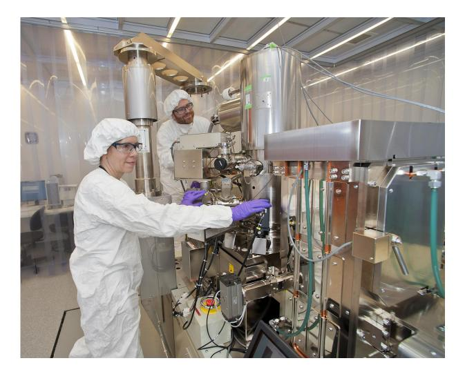
Brookhaven National Laboratory Center for Functional Nanomaterials researchers Gwen Wright and Aaron Stein are at the electron beam lithography writer in the CFN cleanroom. Credit: Brookhaven National Laboratory
