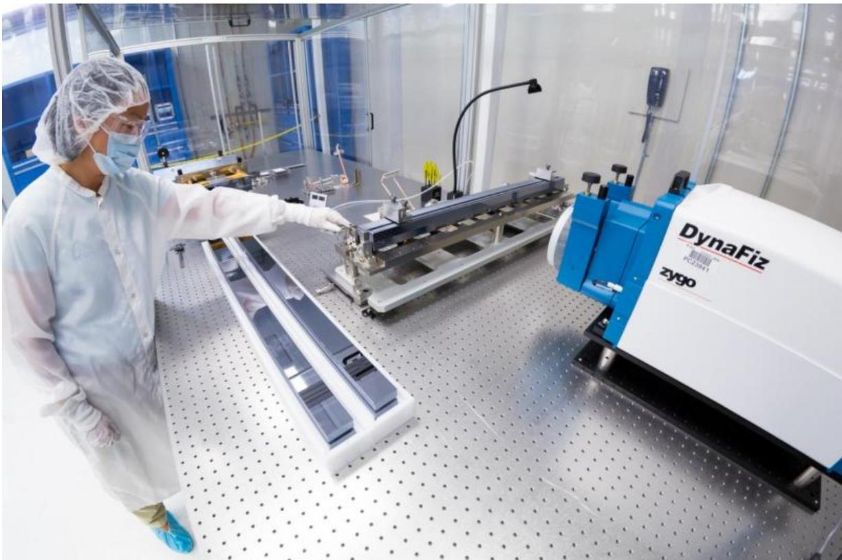
May Ling Ng, SLAC engineer, makes adjustments to the mirror restraints during a test of the holding system's effect on mirror shape. These measurements are needed to maintain the flatness of the mirror within one atom over the entire one-meter length. Credit: SLAC National Accelerator Laboratory
