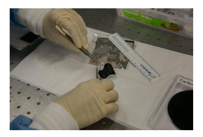
Ngoc Bui demonstrates the flexibility of a carbon nanotube membrane. Credit: Lawrence Livermore National Laboratory
