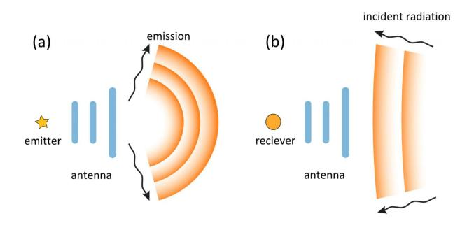
Electromagnetic antenna in transmitting (a) and receiving (b) modes. Credit: Moscow Institute of Physics and Technology
