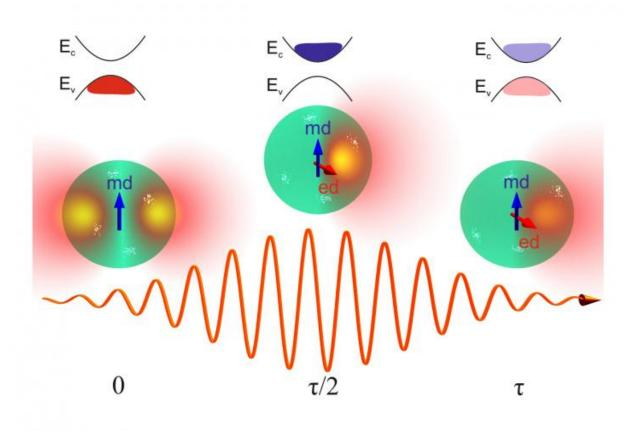
Schematic representation of the system studied in the paper. Photoexcitation of a silicon nanoparticle by a femtosecond laser pulse. Intense irradiation excites electrons in the silicon nanoparticle into the conduction band, which alters the optical properties of the particle (amplitudes of electric and magnetic dipole resonance) in a way that enables unidirectional scattering of incident light. Credit: Moscow Institute of Physics and Technology
