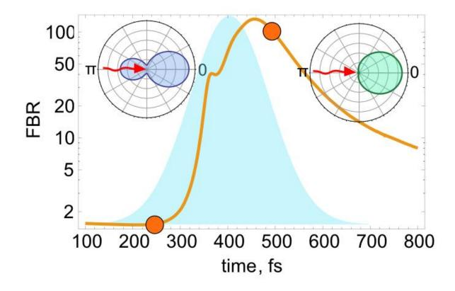
This graph shows the front-to-back ratio (FBR) of a nanoparticle, i.e. the ratio of the power transmitted in the forward direction to the power transmitted in the backward direction. The light blue shaded area in the background represents the envelope of the pulse intensity. The two insets contain the scattering diagrams of the antenna for two different times with the red arrows representing the incident beam. Credit: Moscow Institute of Physics and Technology
