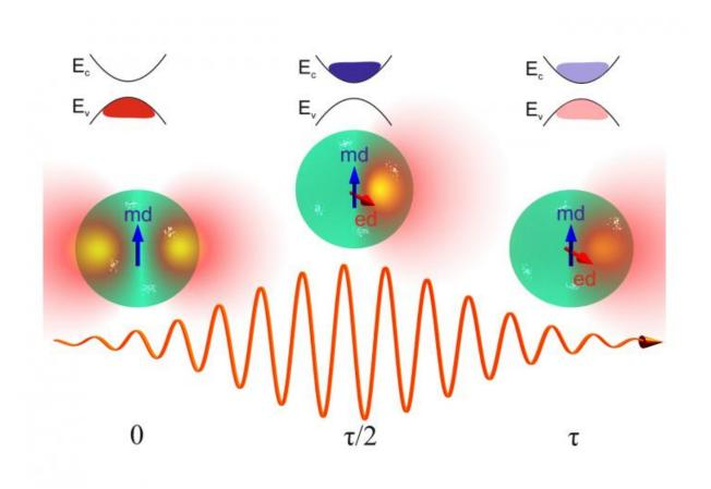
Schematic representation of the system studied in the paper. Photoexcitation of a silicon nanoparticle by a femtosecond laser pulse. Intense irradiation excites electrons in the silicon nanoparticle into the conduction band, which alters the optical properties of the particle (amplitudes of electric and magnetic dipole resonance) in a way that enables unidirectional scattering of incident light. Credit: Moscow Institute of Physics and Technology
