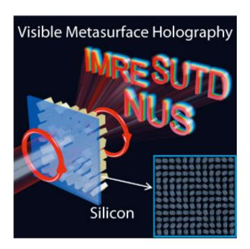
Circularly polarized light passed through silicon nanorods creates a multilayer image. Lower right inset: SEM image of the material. Credit: WILEY-VCH Verlag GmbH & Co. KGaA, Weinheim
