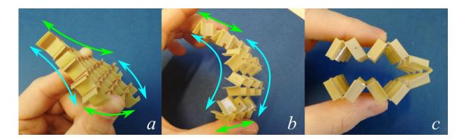
Bending behavior. (a) Synclastic curvature in the closed configuation; (b) cylindrical curvature in the open rec configurations; (c) an open rec specimen folder double. Credit: University of Bristol
