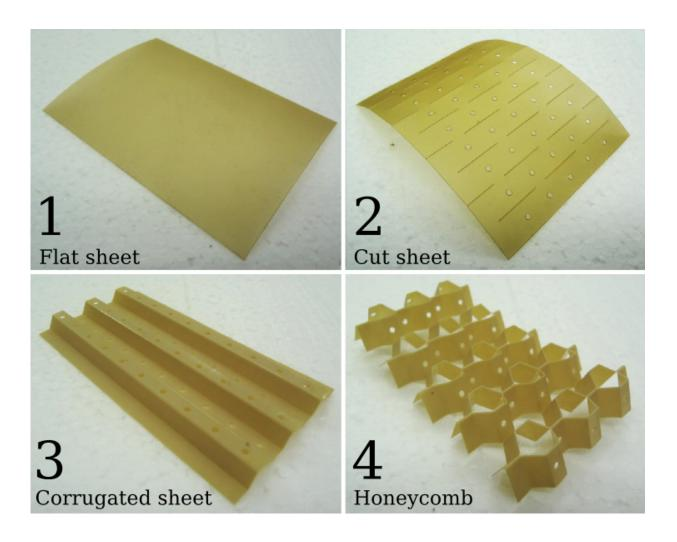
An open honeycomb at each stage during the manufacturing process. Credit: University of Bristol
