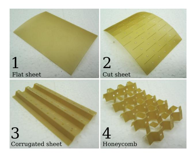
An open honeycomb at each stage during the manufacturing process. Credit: University of Bristol
