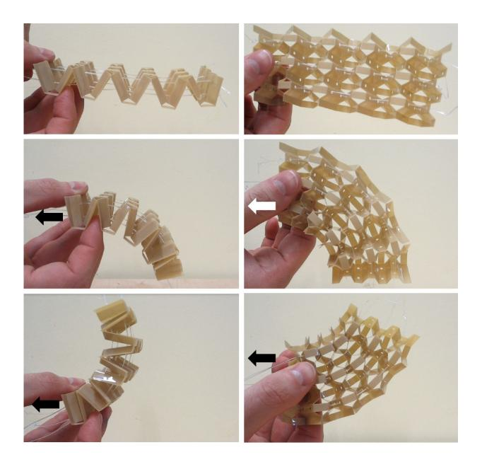
A demonstrator honeycomb changing shape in response to cable tension. The arrows indicate which cable is being pulled Credit: University of Bristol
