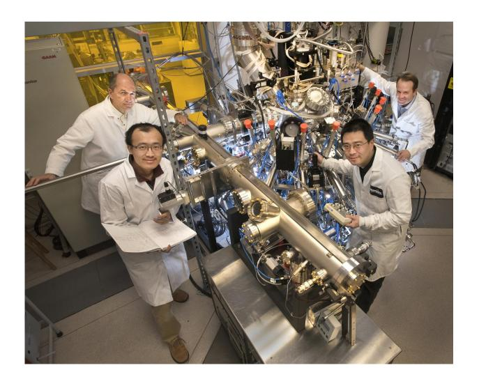
(Clockwise from left) Brookhaven Lab physicists Ivan Bozovic, Anthony Bollinger, and Jie Wu, and postdoctoral researcher Xi He are with the atomic layer-by-layer molecular beam epitaxy system used to synthesize more than 2,500 thin films of a copper-oxide compound called LSCO. The team studied LSCO to understand why it can become superconducting at a much higher
