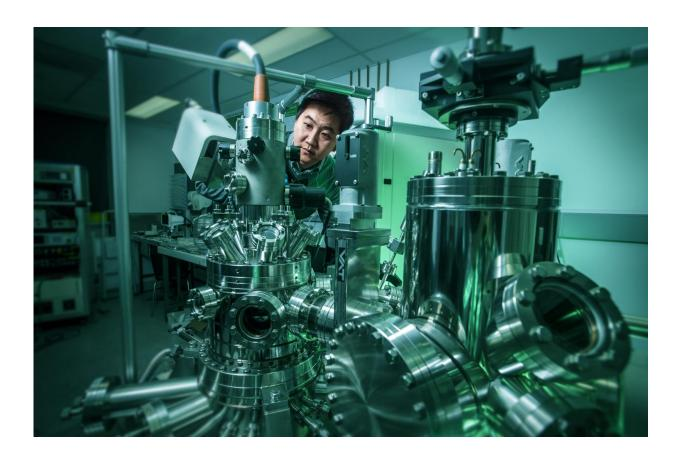
Dr Yi Du and his team's work involves several special techniques that can be done only at ISEM with the help of its powerful tools, including a scanning tunneling microscope, which creates an ultra-high vacuum environment about a hundred times higher than the vacuum level experienced in orbit at the International Space Station. Credit: University of Wollongong
