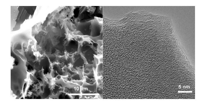
High-resolution transmission microscope (left) and scanning electron microscope images of a porous carbon sample studied for its ability to capture carbon dioxide from natural gas. Credit: Barron Research Group/Rice University
