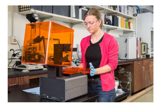
Dulcie Head loads a tray of resin into the 3-D printer that she and Professor Tiziana Vanorio used to create physical models of digitally scanned rock samples. Credit: L.A. Cicero
