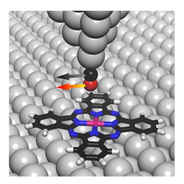
The tip of a scanning tunneling microscope (top center), to which a single carbon monoxide molecule (red and black spheres) has been attached, is scanned in the direction of the arrows over a single cobalt phthalocyanine molecule. Credit: US Department of Energy
