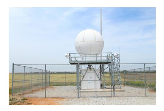
Several X-band scanning precipitation radars are located throughout the Atmospheric Radiation Measurement (ARM) Climate Research Facility's Southern Great Plains site. They are dual-polarized Doppler weather radars for measuring precipitation type and rainfall rates. Credit: US Department of Energy
