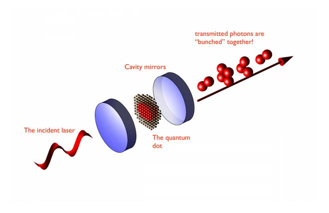
Between two mirrors, the quantum dot filters the light beams with just one photon per package out of the laser, so that only packages with multiple photons remain. Credit: Leiden Institute of Physics
