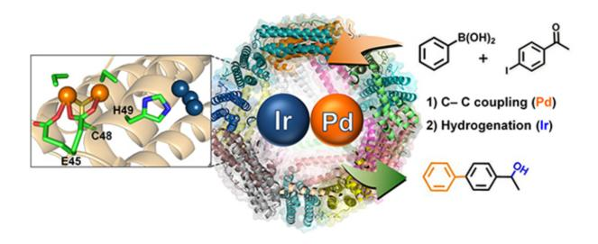
Schematic representation showing the crystal structure and catalytic reactions of apo-ferritin cage containing both Ir and Pd complexes. Credit: Tokyo Institute of Technology
