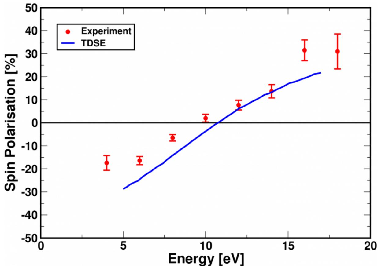
Fig. 1: Spin polarization measured as a function of electron energy. The blue curve is a theoretical prediction, while the red dots with error-bars show experimental results. The measurement was done for Xe atom. Credit: MBI
