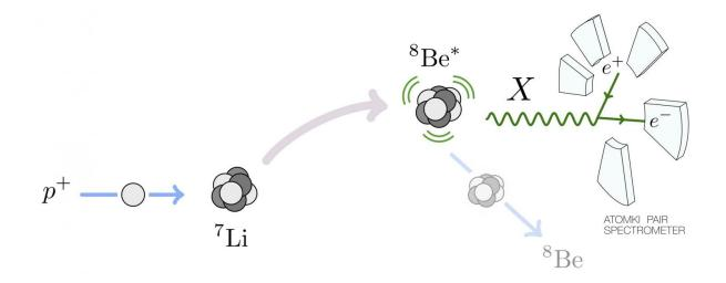
A schematic description of the experimental anomaly that Tanedo and his colleagues have investigated. Excited beryllium-8 nuclei can decay into their ground state while emitting electron-positron pairs. The results of the experiment suggest the presence of a new force particle, here labelled as X. Credit: UC Riverside
