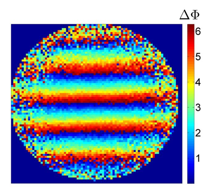
NIST's compact gyroscope measures rotation by analyzing patterns of interfering matter waves in an expanding cloud of atoms transitioning between two energy states. Each atom's speed determines both its final position in the cloud and the
