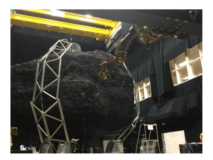
In the Robotics Operation Center at NASA's Goddard Space Flight Center in Greenbelt, Maryland, an engineering development unit of the robotic capture system is tested at full scale. Credit: NASA
