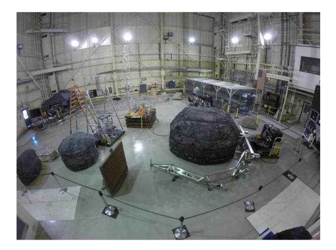
In the Spacecraft Structures Lab at NASA's Langley Research Center, Asteroid Redirect Mission robotic contact and restraint system is prototyped and tested. Credit: NASA
