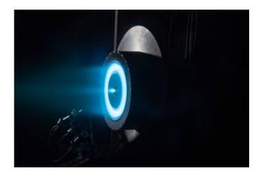
The HERMeS (Hall Effect Rocket with Magnetic Shielding) Technology Development Unit thruster exceeds over 1300 hours of operational wear testing in a vacuum facility at GRC. Magnetic shielding protects the walls of the thruster from erosion, a major breakthrough in Hall thruster design that could hold the key to long-life, reusable electric propulsion systems. Credit: NASA
