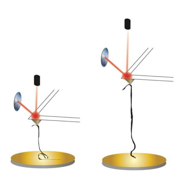
The tip of an atomic force microscope on a cantilevered arm is used to pull a graphene nanoribbon the same way it would be used to pull apart a protein or a strand of DNA in a Rice University lab. The microscope can be used to measure properties like rigidity in a material as it's manipulated by the tip. Credit: Kiang
