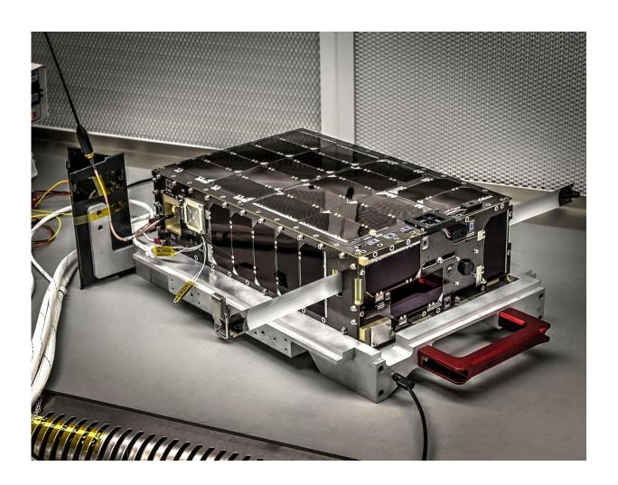
Dellingr's exterior is lined with solar panels. Slighty larger than a cereal box, Dellingr is a six-unit, or 6U, CubeSat -- indicating its volume is approximately six liters. Credit: NASA's Goddard Space Flight Center/Bill Hrybyk
