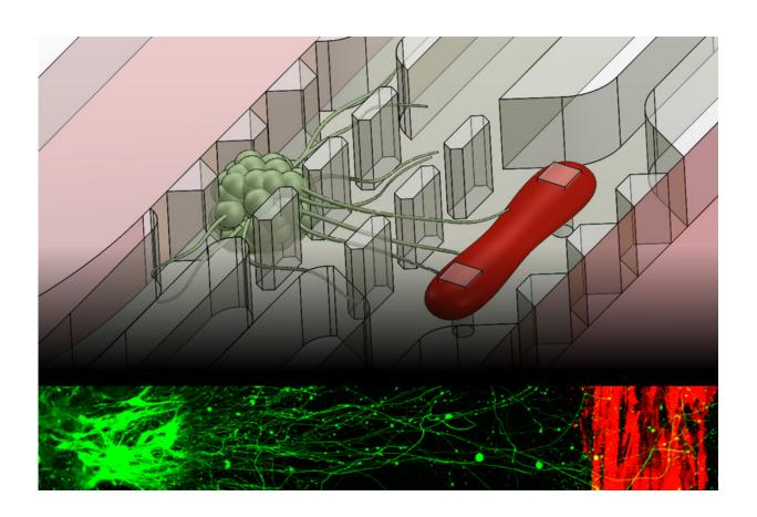
A new microfluidic device that replicates the neuromuscular junction — the vital connection where nerve meets muscle — contains a small cluster of neurons (green) and a single muscle fiber (red). A fluorescence image, bottom, shows the motor neurons sending out axons toward a muscle strip over a distance of about 1 millimeter. Credit: Sebastien Uzel
