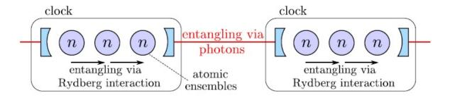
Schematic of two entangled atomic clocks that are part of a larger entangled network of clocks. Each clock here consists of three ensembles, with each ensemble containing hundreds of entangled atoms. Entanglement is generated among atoms within each ensemble, then between ensembles in the same clock, and then between clocks. Credit: Kómár et al. ©2016 American Physical Society
