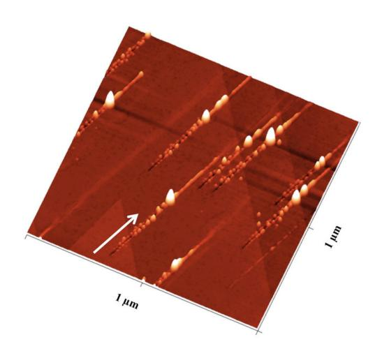
Nanostructures on a crystal after ion bombardment: Trenches with nanohillocks on either side are created. At the impact site, a particularly large nanohillock is formed. Credit: Vienna University of Technology
