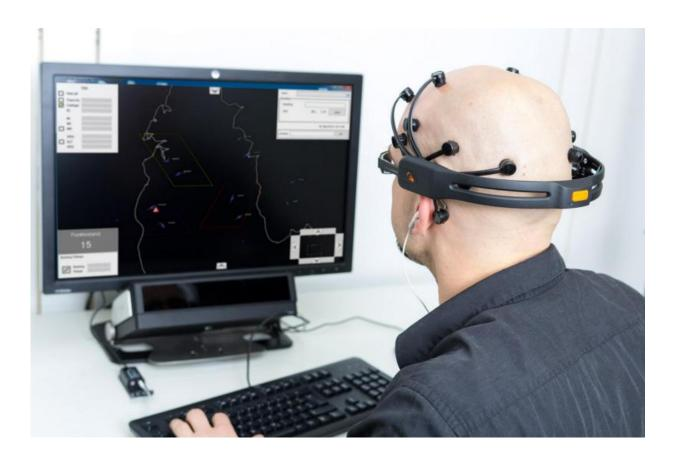
The interaction of man and machine is particularly important for air traffic controllers. A software from Fraunhofer FKIE assesses user states and human performance and passes this information on to the computer. Credit: Fraunhofer FKIE
