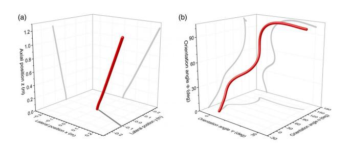
Figure 6 in the article shows trajectory of (a) position and (b) orientation of pliers under repetitive laser irradiation without tracking. Grey lines indicate the projections of the trajectory in the respective coordinate planes. Credit: © the authors doi:10.1117/1.OE.56.1.011007.
