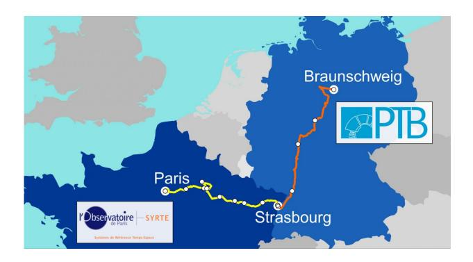
Metrological optical fiber link between LNE-SYRTE in Paris, France and PTB in Braunschweig, Germany, connected in Strasbourg. The overall link length is 1400 km. Credit: Physikalisch-Technische Bundesanstalt
