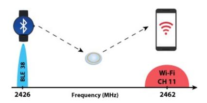
In interscatter communication, a backscattering device such as a smart contact lens converts Bluetooth transmissions from a device such as a smartwatch to generate Wi-Fi signals that can be read by a phone or tablet. Credit: University of Washington
