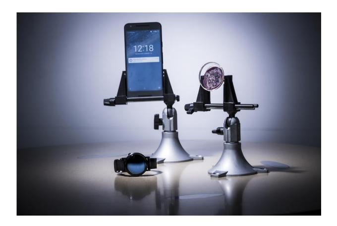
"Interscatter" communication generates low-power Wi-Fi transmissions using everyday mobile devices. In one example, Bluetooth signals from a smartwatch (left) were used to transmit data from a neural device that can be implanted in a patient's brain (right) to a smartphone via Wi-FI. Credit: Mark Stone/University of Washington
