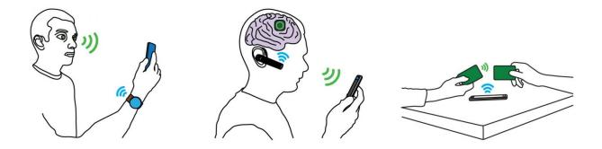
Examples of interscatter communication include a) a smart contact lens using Bluetooth signals from a watch to send data to a phone b) an implantable brain interface communicating via a Bluetooth headset and smartphone and c) credit cards communicating by backscattering Bluetooth transmissions from a phone. Credit: University of Washington
