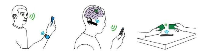
Examples of interscatter communication include a) a smart contact lens using Bluetooth signals from a watch to send data to a phone b) an implantable brain interface communicating via a Bluetooth headset and smartphone and c) credit cards communicating by backscattering Bluetooth transmissions from a phone. Credit: University of Washington
