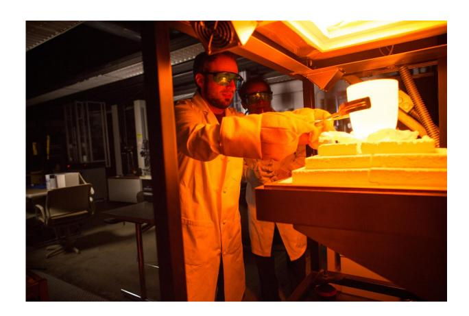
As part of his doctoral research, Charles McLaren discovered that applying a direct current field across glass reduced its melting temperature. In their experiments, they placed a block of glass between a cathode and anode, and then exerted steady pressure on the glass while gradually heating it. Credit: Douglas Benedict of Academic Image
