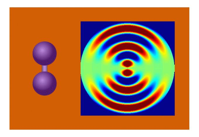
The electron diffraction pattern from iodine molecules depends on the distance between the two iodine nuclei, and changes as the molecule vibrates. Credit: SLAC National Accelerator Laboratory
