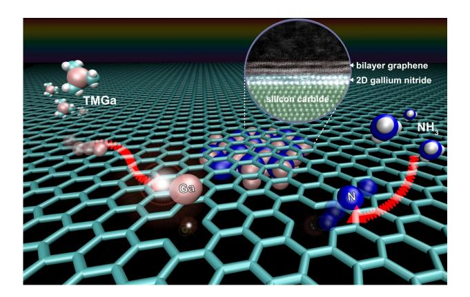
An illustration of the Migration Enhance Encapsulated Growth (MEEG) process to stabilize novel wide-bandgap two-dimensional nitride semiconductors that are not naturally occurring. MEEG is facilitated by defects in the graphene lattice that act as pathways for intercalation. When the gallium and nitrogen adatoms meet at the graphene/SiC interface, they chemically react to form twodimensional gallium nitride. Credit: Z. Al Balushi and Stephen Weitzner, Penn State MatSE
