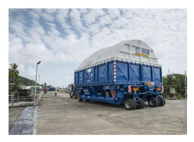
The EPS upper stage of Galileo's Ariane 5 being transferred by road from French Guiana's Pariacabo Port to Europe's Spaceport on 22 August. Credit: ESA-CNES-Arianespace/Optique Video du CSG/Jourrenberger
